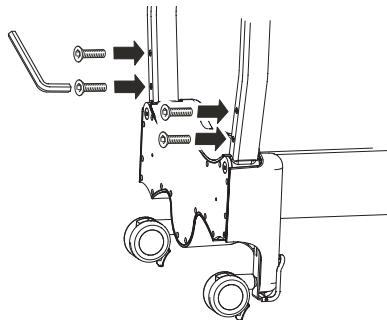
4. Insert the curved boom section into the boom carriage. Secure the assembly by inserting the two 6mm countersunk screws into the blue capping plate provided in the fastener kit, as shown below and tighten firmly.
