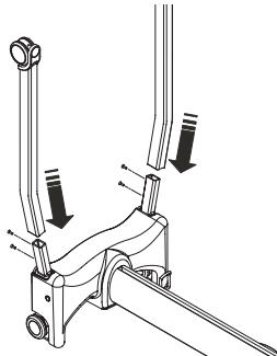
3. Using Allen Key provided, tighten the 6mm screws located on each side of the chassis.
