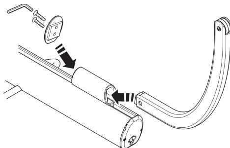
5. Attach four point positioning cradle to the lift boom by inserting the split pin. Ensure pin is secure.
