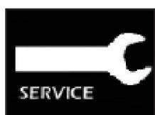
When it is time for a service, the service symbol will appear on the display. In addition, when the user handset is activated, the Smart Monitor will give an audible signal giving notice to users that a service is required.
